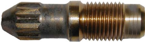
Hot runner nozzle after treating with micro-abrasive blasting
