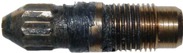
Hot runner nozzle encrusted with residue build-up
