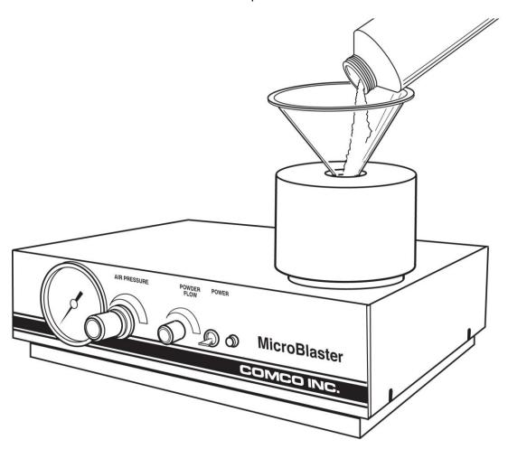
Figure 3-3: Filling the Abrasive Tank
