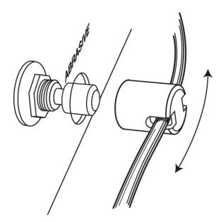
Figure 4-1: Pinch Tube and Plunger Inspection
