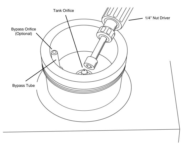
Figure 3-1: Changing the Tank Orifice
