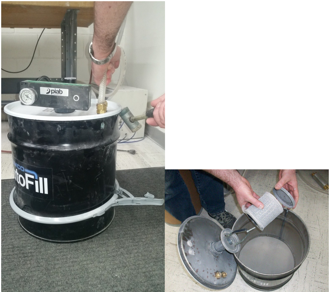
Figure 4 – Opening the Vacuum Generator and accessing the HEPA filter
